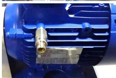
EXEMPLE DE MONTAGE DU KIT MBP013 INTÉGRÉ DANS NOTRE BANC MTR100
