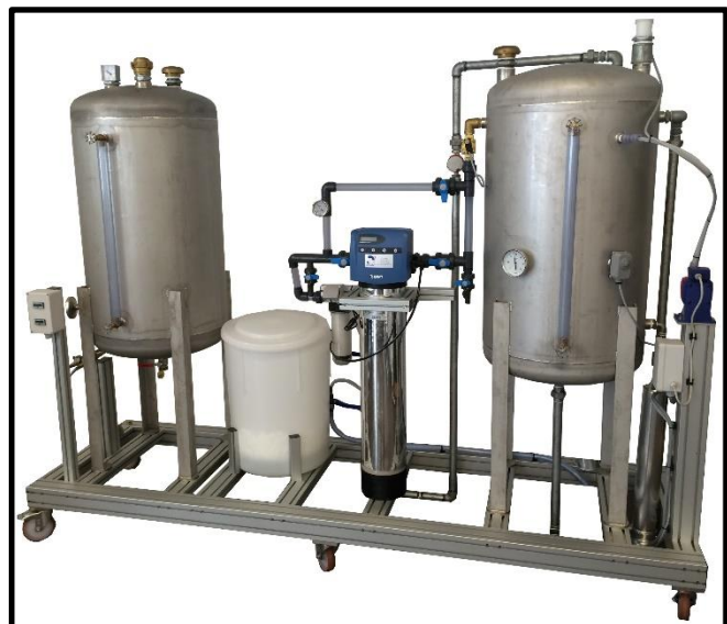
Water tank (hotwell), softener and fuel tank
